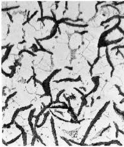
Gray iron \alpha Fe and graphite flakes
