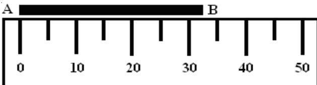
You are measuring the length of the object AB. You have kept end A exactly in line with the graduation 0. Assume also that the length is kept parallel to the edge of the scale. You may have a tendency to read the length as 32 or 32.5. It is wrong. You are expected to read it either as 30 or as 35. You may mention the error like  $30^{+5}$  or  $35^{-5}$ . This is applicable not only to length measurement, but to all analogue displays; you must not read between the lowest two divisions.
