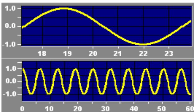
Check for the best identifiable zero crossings towards the left end and the right end; measure the total time and count the number of cycles; total time divided by the number of cycles gives the period. Whatever small error is there in identifying zero crossing gets divided by the number of cycles used; larger the number of cycles better the accuracy. Note that the error contributed by the resolution of the scale remains the same whether you take one cycle or 10 cycles!
