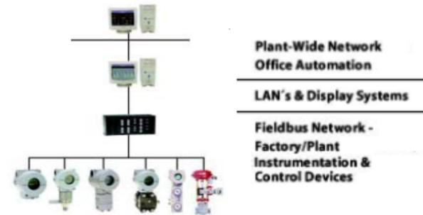
**Fieldbus** can also be seen as the family of industrial communication protocols used for real-time distributed control, now standardized as **IEC 61158**. Devices can be networked and configured according to the user needs. The system is fully scalable in the sense that it can be implemented for small plants to large plants.
